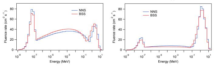
Figure 5: The neutron spectra, measured by the NNS and BSS, of bare (right) and moderated (left) Californium-252. Both tests were conducted at the Health Physics Neutron Generator facility in Chalk River, Canada [1].
