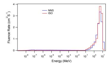
Figure 2: AmBe neutron spectrum as measured by the NNS and compared to the ISO standard spectrum. These measurements were conducted at the low scatter facility in the Ionizing Radiation Standards Laboratory of the National Research Council of Canada (IRS-NRC) [1].
