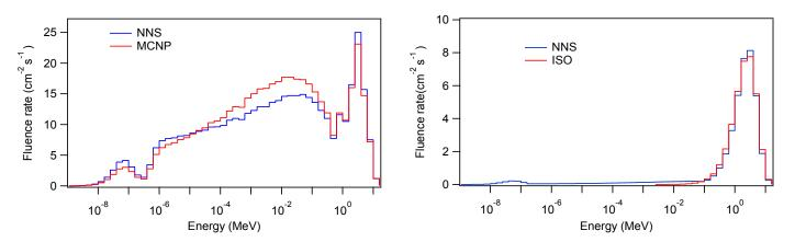
Figure 1: The neutron spectra of bare (right) and moderated (left) Californium-252 as measured by the NNS. For comparison the ISO/NIST standard spectrum is included. Both tests were conducted in the low scatter facility at the National Institute of Standards and Technology (NIST) in the United States [1].
